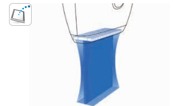
Figure 2 intelligent Dynamic Micro-Slice (iDMS) technology provides high-flexibility electronic focusing in the lens direction and improves the elevation resolution.
